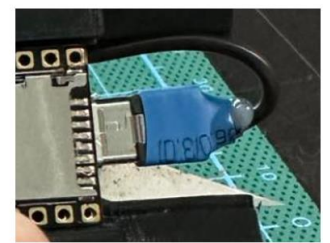
Step 4 – Use a short length of larger heat-shrink tubing over the pad areas
